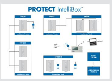
See examples of three different ways of connecting several fog cannon units on the back, all using an IntelliBox controller.
