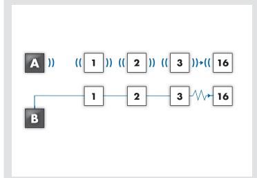
Each IntelliBox can control up to 16 fog cannon units. Depending on the security class required, you either choose a wireless connection (A) or a cabled connection (B) - or a combination.
