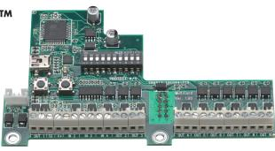
Add various useful functionalities to the fog cannon. E.g. 9 extra output signals for precise and separate identification of the output signals. And input for reliable and simple panic button solution. MultiCard saves end users and installers valuable time and money during, and after installation.
