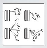
For most of our fog cannons you can choose between four different nozzles: straight forward, 30 degree, 3-hole and combined 3-hole/30 degree.
