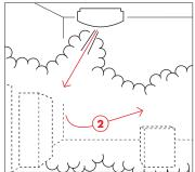
The direction and deployment of the fog in point protection is illustrated with the arrows. After the first, instant protection of the most valuable items (1) the fog spreads to the rest of the room (2). Walls and floors effectively make the fog "bounce" in all directions.
